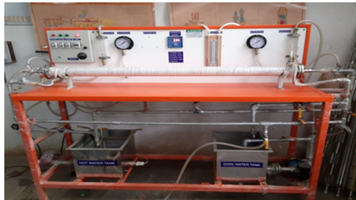
Figure 8: Double Pipe Heat Exchanger with Interrupted Fins
